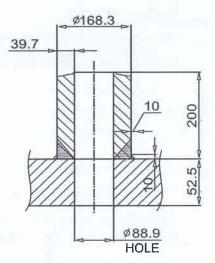
For the above configuration, confirm whether compensation is required and if compensation check is required, confirm whether the configuration satisfies the compensation requirements. (Assume ligament efficiency of shell as 100%)
